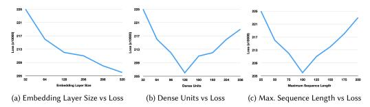
Fig. 7. Sensitivity of PACS to hyper-parameters; (a) Embedding Layer size, (b) Dense units, and (c) Maximum Sequence Length.
