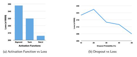
Fig. 6. Sensitivity of PACS to hyper-parameters; (a) Activation function and (b) Dropout probability.
